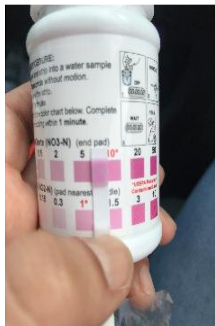
Figure 1. A nitrate test strip held against the calibrated colour switch to assess drainage water nitrate concentration.
