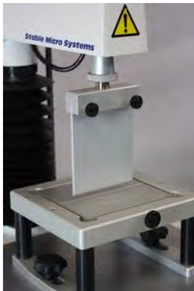
Cutting blade with guillotine edge (Blade 11054, 90 mm height, 70 mm width, 3 mm thickness)
